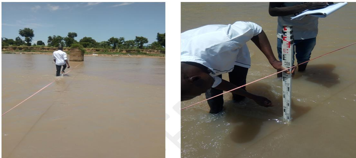
Plate 1: Methods of determining the width and depth of channel
